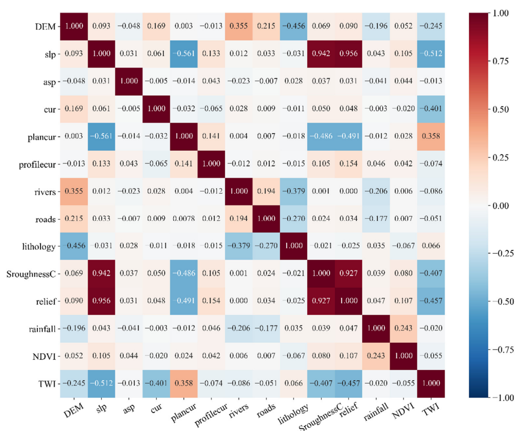
Figure 8. Pearson correlation coefficient matrix for the Wuqi County case study. Note that “slp” represents slope, “asp” represents aspect, “cur” represents curvature, “plancur” represents plane curvature, “profilecur” represents profile curvature, “rivers” represents distance to rivers, “roads” represents distance to roads, “lithology” represents lithology, “SroughnessC” represents surface roughness, “relief” represents relief amplitude, and “rainfall” represents rainfall.
